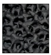
Filter Sleeves use advanced ceramic foam filters available for most metal types. Standard pore sizes include:
