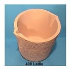
Joy-Mark manufactures ladles with both an ID and OD forming process. The 409 ladle shown at left is an ID formed part, which maximizes density inside the ladle to resist metal penetration and ladle erosion. The 409 also features a double pouring lip configuration. Single lip configurations are also available. The ID formed style is an excellent choice as a ladle liner. They are available in a wide range of capacities (see table on back page). OD formed ladles may also be used as ladle liners.
