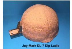
The DL-6.5 and DL-7 (shown at the left) have a large capacity and has a heavy duty "L-bracket" for secure attachment. The bracket is 2-1/4" wide, with two 7/16" mounting holes, and protrudes 4" from the ladle.
